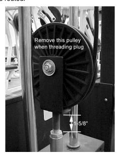
Figure 12. Bolt the floating pulley into the 190 lb weight stack (away from the tricep pushdown weight stack).
